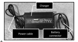
In a wet environment, there is a risk of creating electric arcs when charging the vehicle. The battery charger is not humidity-proof.
