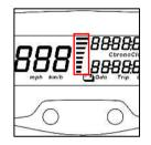
The battery charge indicator is composed of 8 bars indicating the range of the motorcycle.
