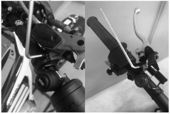
For the lever positioning, you have to adjust these 2 screws.
