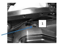
Open the drain plug 2 Be careful: the oil will flow, install an oil container
