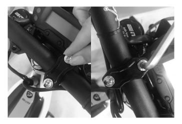
Please, frequently check that the screws holding the handlebars on the bar mounts are tight.
