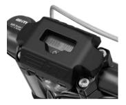
The battery level indicator goes in sleep mode after 10 second, to display again the battery percentage level, you have to push the main button located directly on the center of the display.
