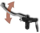
But this lever can also be used as PRB (Progressive Regenerator Brake). When the pilot is not accelerating, the motor is not powered. If it is in freewheel, it is possible to regenerate the motor ; it allows to recharge the battery while acting as a motor brake. Therefore, this lever allows to manage the regeneration percentage.
