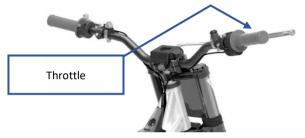
Before each use, check that the throttle grip rotates and returns correctly to prevent any accident.
